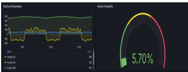
Fig. 4. Electrical Parameters vs. Failure Probability
